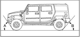
The HUMMER H3 has an approximate approach angle (A) of 37.5 degrees and a departure angle (B) of 35.5 degrees, depending on suspension packages.
